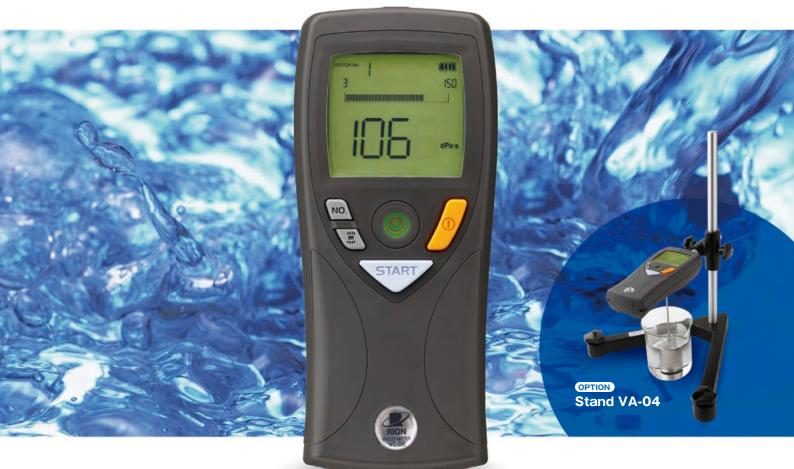
The VT-06 is designed for quality control applications in the manufacturing process of industrial products such as petrochemicals, paint, and adhesives, as well as foodstuffs. Viscosity measurements covering a wide range are possible, such as gear oil used in construction machinery. Measurement is performed by simply submerging a rotor in the fluid. The resistance to rotor movement caused by the viscosity (torque) is measured to obtain direct readings.
