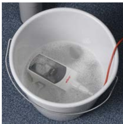
TF 410 - still working, thanks to IP67
