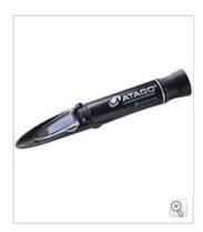
This instrument measures the salinity and specific gravity of seawater, and utilizes a new material that is durable against salty samples, The salinity of seawater is displayed in parts per mill (‰). It is an Automatic Temperature Compensation (ATC) model with water resistant properties (IP65).
