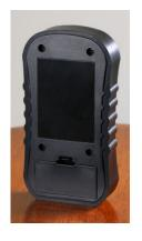
\*Although not recommended, you may wish to use the meter without the protective rubber boot. If you choose to do so, make sure you recalibrate your meter on the On-Demand Calibrator with the boot off.
