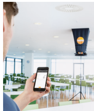
App integration via Bluetooth for displaying the measurement data on mobile devices and finalizing the measurement report on site.
