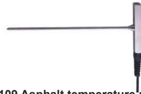
No. 8250-68 MC-K7109 Asphalt temperature probe Range: 0 to 300°C (class 2), Ø5 x 250 mm (point-end) Cord length: 1.5 m
