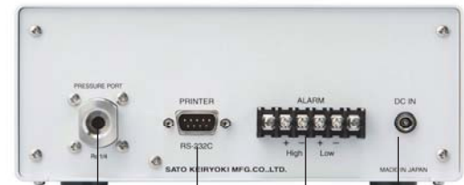
Pressure port: Rc1/4 RS-232C/Printer output Alarm output port (upper and Lower) AC adapter connection port
