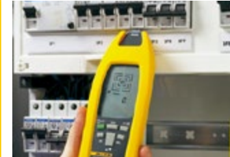
Location of fuses/breakers and assignment to circuits
