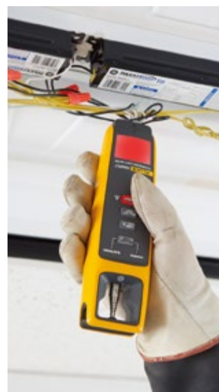
Non-contact voltage: Quickly check for voltage presence
