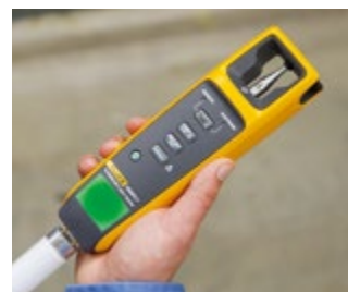
Pin continuity test: Test if filaments have continuity
