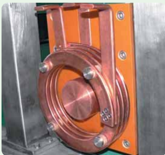
▲ Coil & Contact, Multi Magnetization
