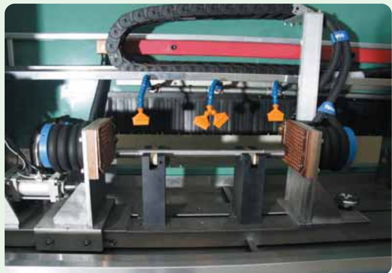
▶ 대형볼트자분탐상기 / PICO-MAG 3000 Contact, Coil, Multi-magnetizing
