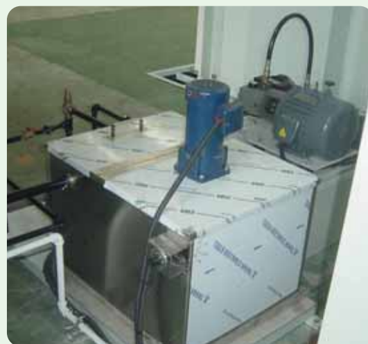
▲ Magnetic Particle Tank & Circulation pump
