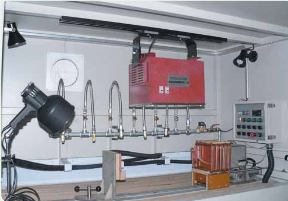
▲ Shaft Inspection 4000 Contact, Coil, Multi-magnetizing
