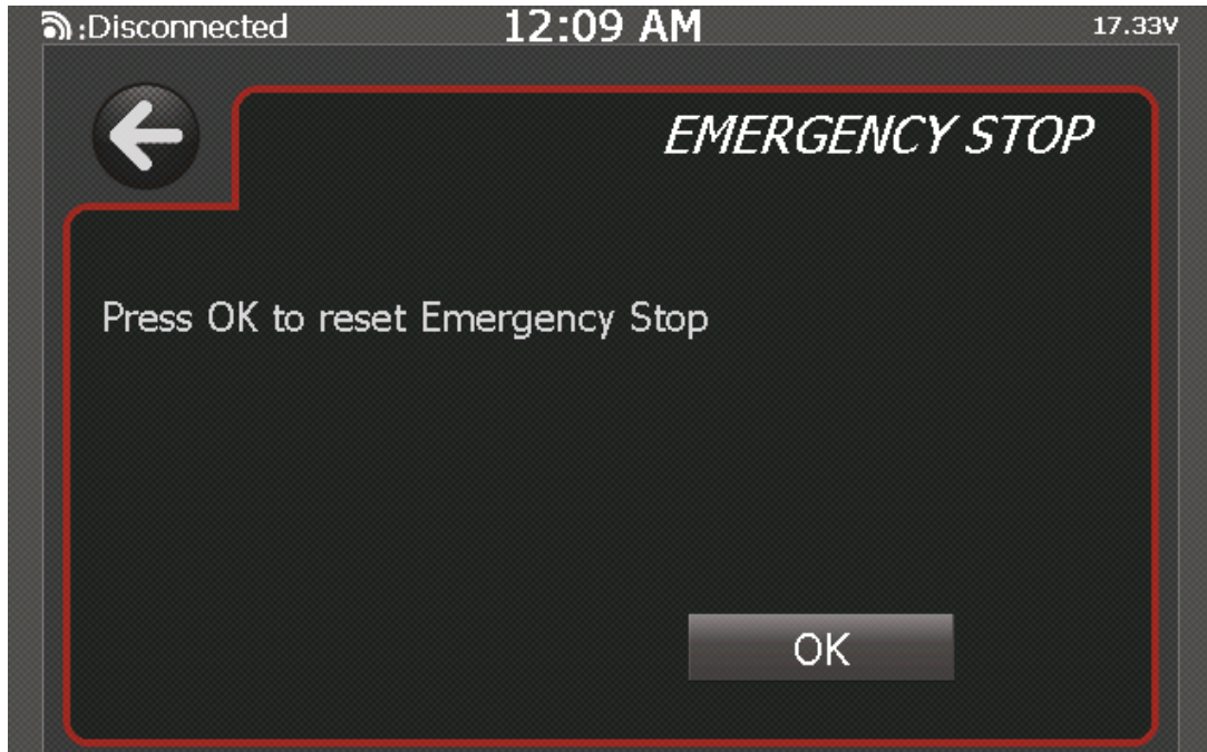
Figure 2.11.3. MDT-2 following emergency stop after power has been turned off and on again.
