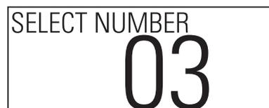
[Note] [01] is reserved for the base calibration curve and cannot be used for user calibrations.
