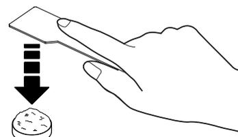
(3) Use the spoon with spatula to level off the sample to the height of the edge of the sample platter.
