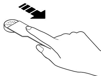
**[Note]** An accurate measurement cannot be taken if there are cracks or lumps in the surface of the sample. Use the spatula to make the surface as flat and smooth as possible.
