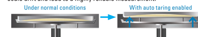
The sample dish rises once per 30 seconds and scale drift is reset.
