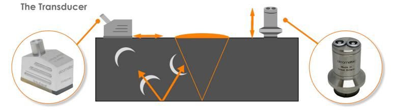
The transducer frequency and diameter will change depending on the size and type of weld and base material. Please see below an example of transducers for a general weld inspection:
