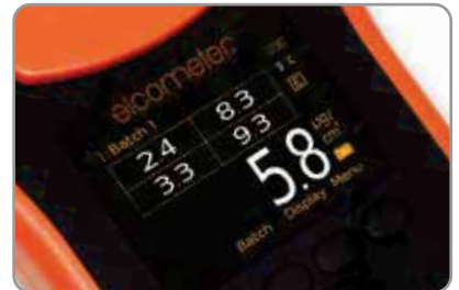
Four Bresle Patch Equivalent Readings
