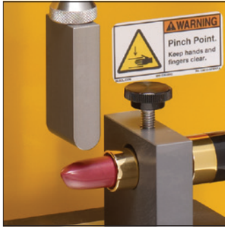
TA-LC Lipstick Cantilever Test Fixture allows imitative tests on lipstick and similar products to quantify strength of product. Fixture Base Table required.
