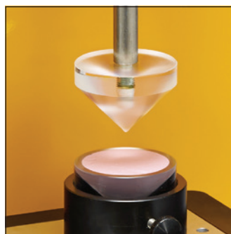
TA-STF Spread Test Fixture quantifies the spread force of a material. Comes with 1 male cone probe, 5 five samples cups and 1 sample cup holder. Base Table required.
