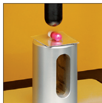
TA-BPS Blister Pack Support Fixture is used to measure the force required to remove the tablet from its blister pack. Fixture Base Table required.
