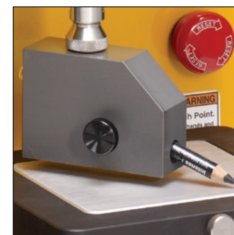
TA-EP Eye Pencil Test Fixture measures hardness of cosmetic pencil tips for eye- or lip-lining products and can also be used for artistic type pencil tips. Fixture Base Table required.
