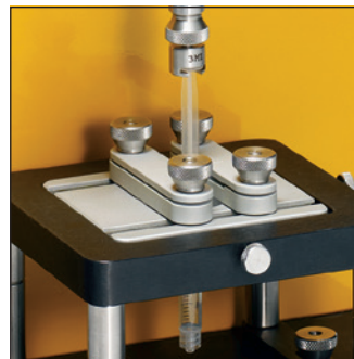
TA-STJ Syringe Test Fixture for measuring the force required to push or pull syringe plunger. Important to all syringe markets. Base Table required.
