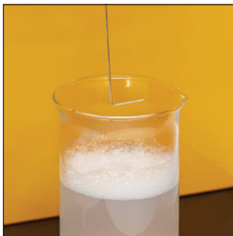
TA-RT Raft Tester measures alginate Raft Strength by pulling wire raft hook out of the sample material.
