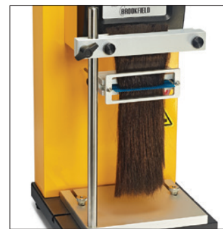
TA-HCF Hair Combability Fixture measures the effect of hair dye, shampoos and conditioners on the combability of hair.
