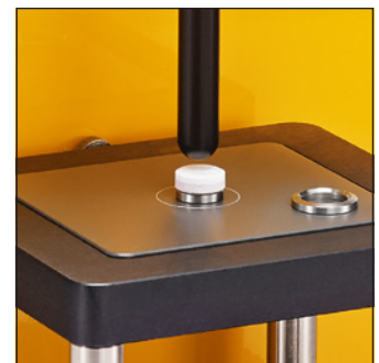
TA-TCF Tablet Compression Fixture performs a ring crush test (includes four rings). Bead compression test fixture is also included. Fixture Base Table required.
