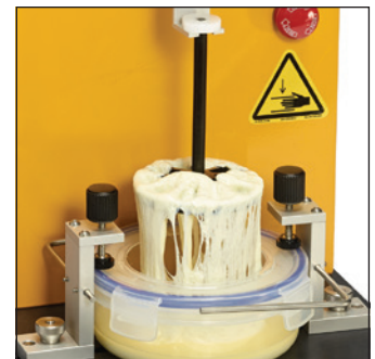
TA-CEF Cheese Extensibility Fixture measures the extensibility of molten cheese sample to breaking point.
