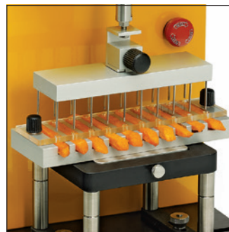
TA-MCF The Multiple Chip Fixture is used for testing the penetration or firmness of multiple chips / french fries. Fixture Base Table required.
