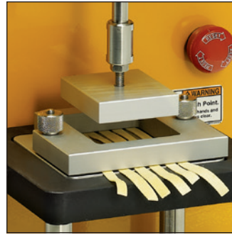
TA-PFS Pasta Firmness and Stickiness Fixture measures the firmness and stickiness of uncooked pasta. Fixture Base Table required.
