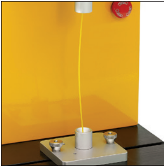
TA-SFF Spaghetti Flexure Fixture quantifies flexure characteristics of uncooked spaghetti and other dry pastas.
