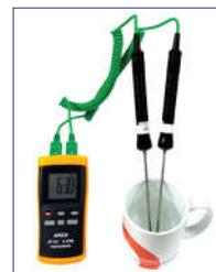
Notice: The thermometer itself can sens or 1370°C, but the test probes can only test the temperature up to - 50 to 204°C, so if you need to test more than 204°C, please change these probes
